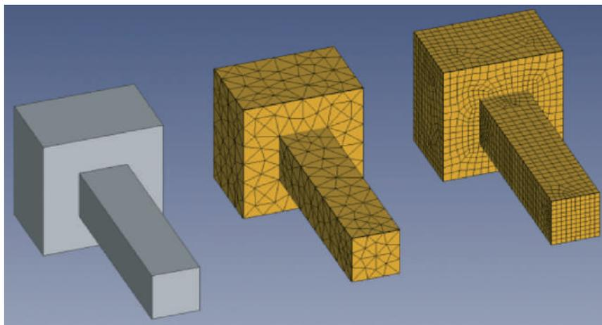
Figure 1 Geometry with tetrahedral and hexahedral meshes (FreeCAD, 2020)
